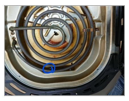
Unscrew the screw keeping the thermal fuse in.
