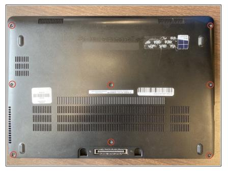
Remove the eight 4 mm screws on the back cover using a Phillips #0 screwdriver.
