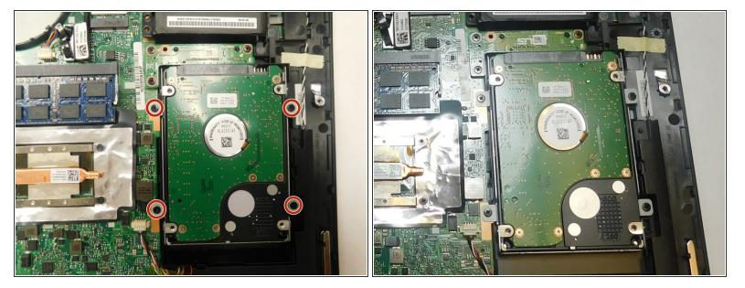
Use a Phillips #0 screwdriver to unscrew the four screws surrounding the hard drive.
