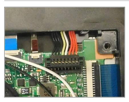
Disconnect the battery connection.
