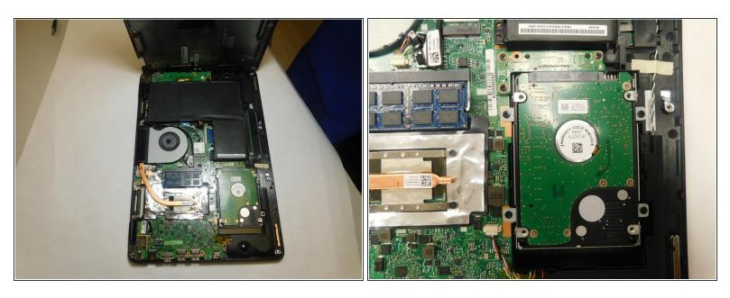
Once you opened the laptop, the hard drive is located on the bottom right from where the battery is.
