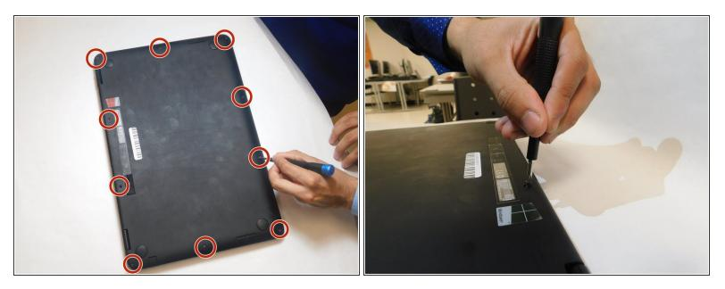
• Remove the ten circled screws along the perimeter of the laptop with a Phillips #0 screwdriver.
