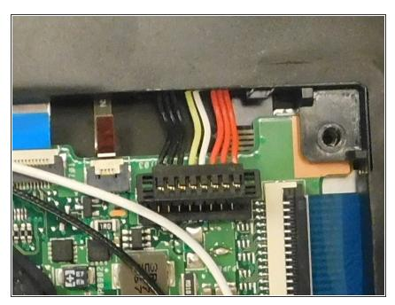
Disconnect the battery connection.
