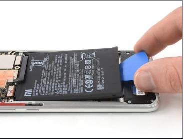
• Use an opening pick or plastic card to pry the battery out of its recess until you can get a good grip.
