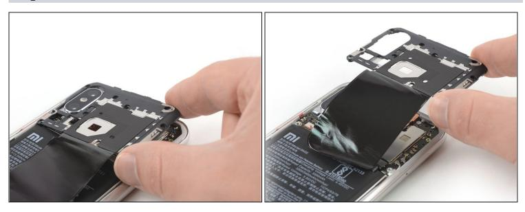
• Carefully remove the motherboard cover including the NFC antenna.
