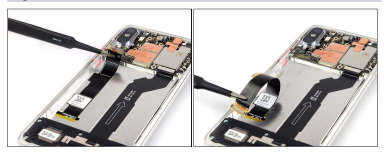
• Use a pair of <u>tweezers</u> to peel the display flex cable off the midframe. It is attached with mild adhesive.
