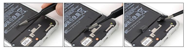
• Use a pair of <u>tweezers</u> to peel the black ends of the adhesive tabs off the battery.
