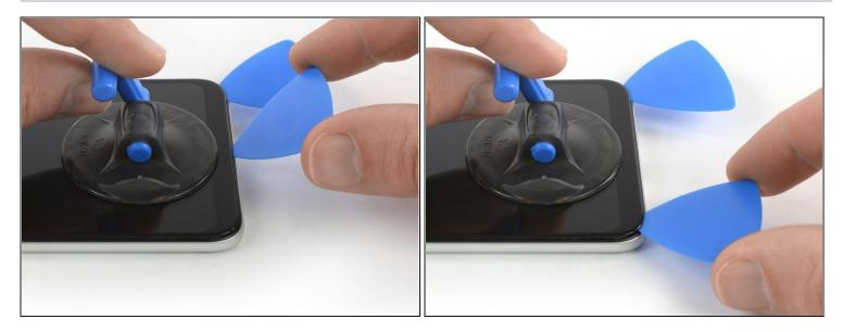
• Insert the tip of a second opening pick and slide it to the bottom left corner of the Xiaomi Mi 8 to cut the adhesive. Leave it there to prevent the adhesive from resealing.
