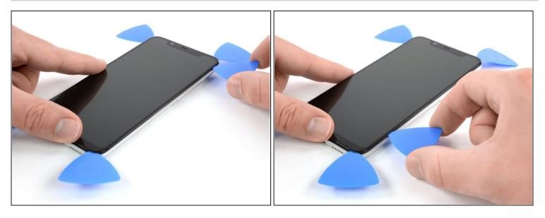
• Insert the tip of a fifth opening pick at the top right corner of the phone and slide it along the right edge to cut the adhesive.
