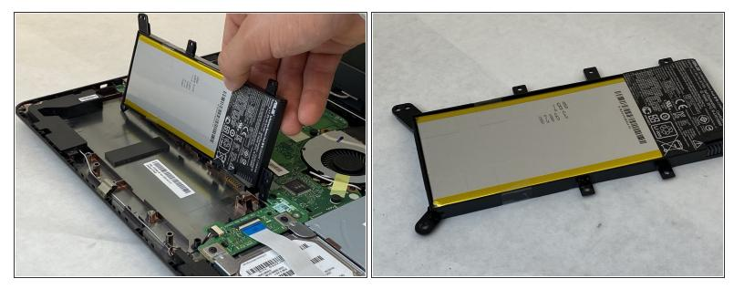
Carefully remove the battery from the device.
