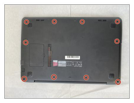
Remove the ten 18 mm screws holding down the outer shell of the laptop using the Phillips #000 screwdriver.
