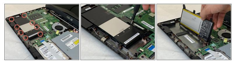
• Use the Phillips #000 screwdriver to remove the eight 4 mm screws holding the battery in place.
