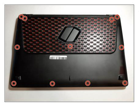
Remove the eleven 6.6 mm screws on the back of the computer using the Phillips #0 screwdriver.
