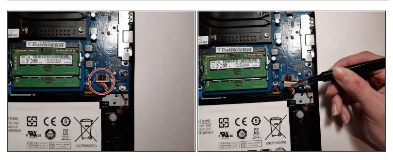
• Disconnect the battery connector cable.
