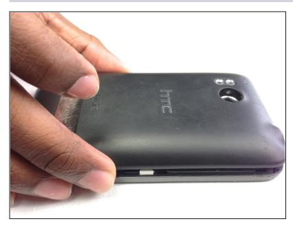
• Lift and remove the rear panel.
