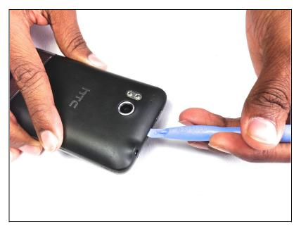
• Insert the plastic opening tool into the top of the Thunderbolt near the power button.
