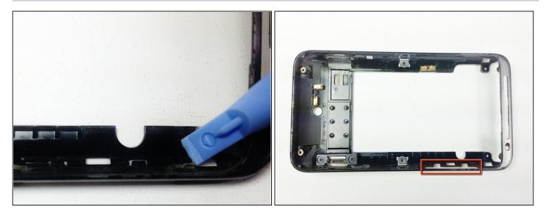
• Use a pry tool to lift the buttons out of the case
