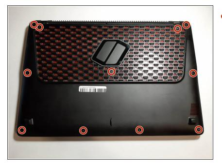
Remove the eleven 6.6 mm screws on the back of the computer using the Phillips #0 screwdriver.
