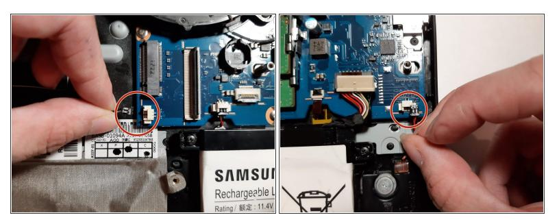
Disconnect the speakers by pulling the plugs out of their sockets.
