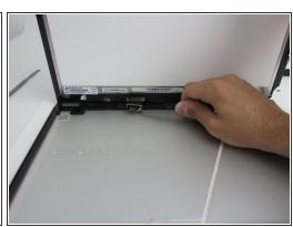
Use tweezers to detach the cables connecting to the back of the screen.
