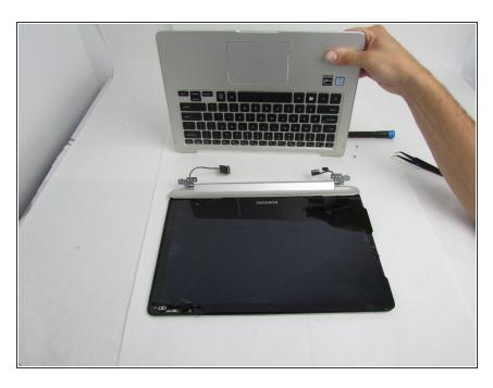
Separate the top and bottom of the computer.
