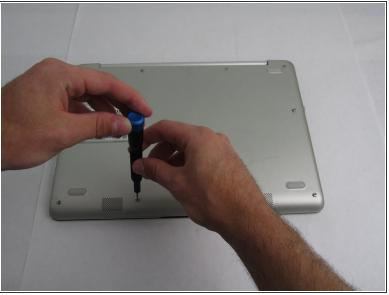
Use a Phillips #00 screwdriver to remove the four 6.5mm screws and the six 4.5mm screws that secure the back plate.
