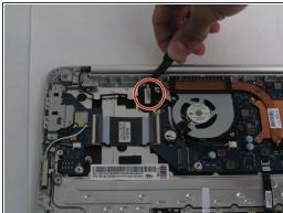
Remove the connections for the screen using a pair of tweezers or your fingers.
