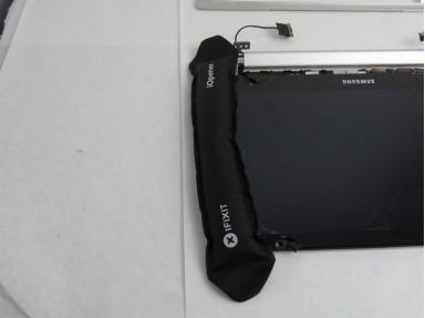
Heat the iFixit iOpener in the microwave for 30-45 seconds and apply it to the edges of the screen to loosen the adhesive.
