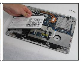
• Use a spudger to pry the battery connecting cable from the laptop and remove the battery.
