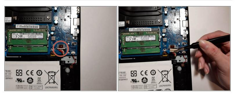
• Disconnect the battery connector cable.
