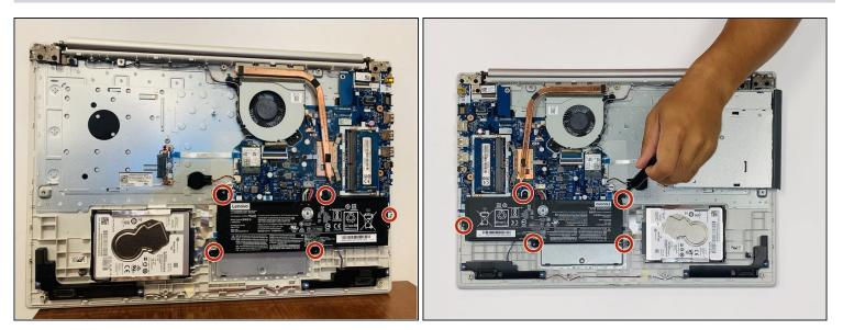
• Remove five 7mm Phillips #0 screws from the battery holder.
