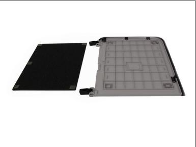
Completely remove the scanner cover by peeling the thin white plastic sheet off.
