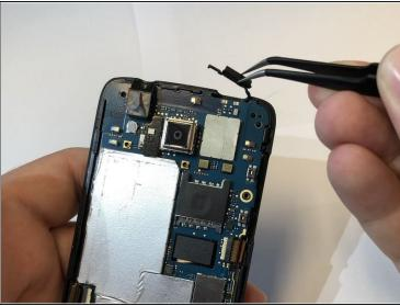
Remove power button from the top of the phone with tweezers.
