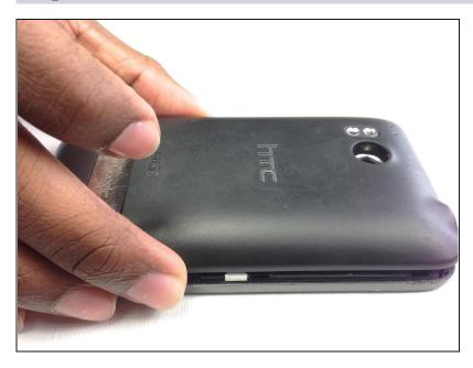
• Lift and remove the rear panel.
