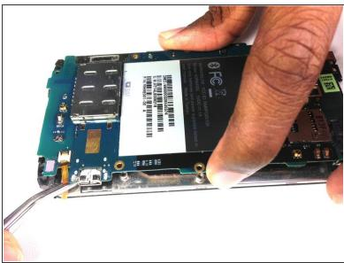
• Using the tip of an plastic opening tool flip up the tab holding the capacitive button ribbon cable.
