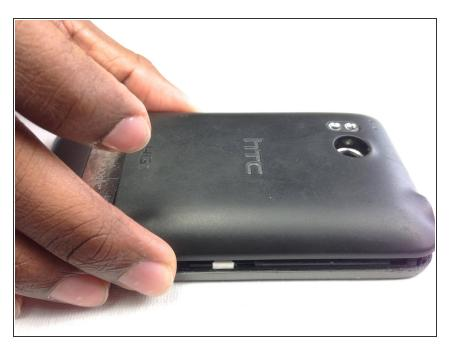
Lift and remove the rear panel.
