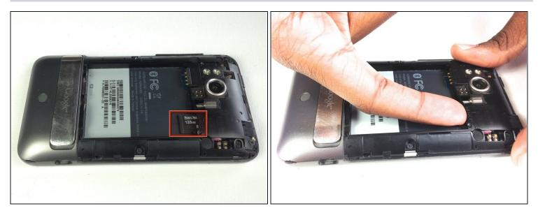
• Use your finger to push the MicroSD card in towards the top of the phone, allowing it to be released from the casing.
