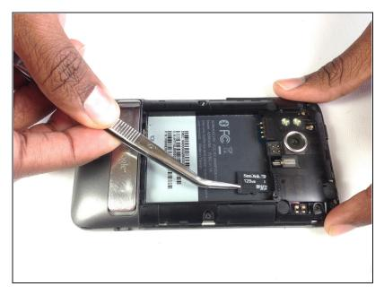
• Use <u>tweezers</u> to grab onto the MicroSD card and carefully remove it from the casing.
