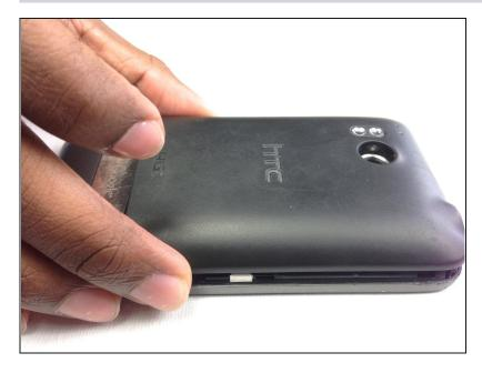
• Lift and remove the rear panel.
