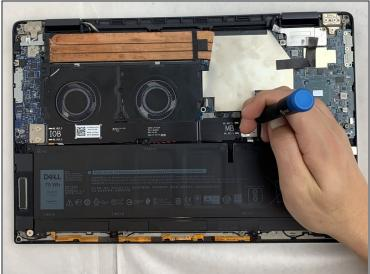
• Use the Phillips #0 screwdriver to remove all four silver 3.2mm screws fastening the interconnect cable.
