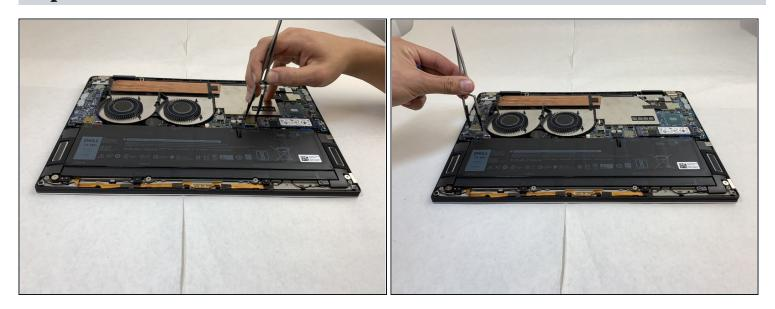
• Use the nylon tweezers to remove the interconnect pins from each of the circuit boards.
