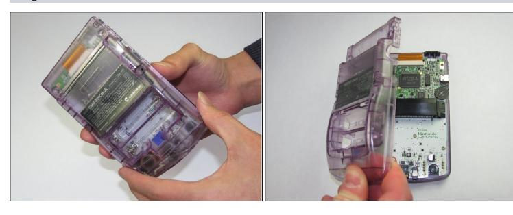
• Gently lift and separate the back housing from the rest of the device. Now you've got the back housing out!
