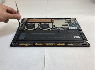
• Use the nylon <u>tweezers</u> to remove the interconnect pins from each of the circuit boards.
