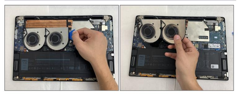
• The fan has been completely disconnected and is now safe to remove.
