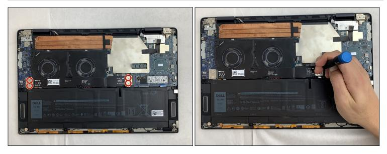
• Use the Phillips #0 screwdriver to remove all four silver 3.2mm screws fastening the interconnect cable.
