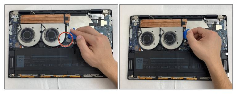
(*i*) Confirm all four screws have been extracted from the fan.
