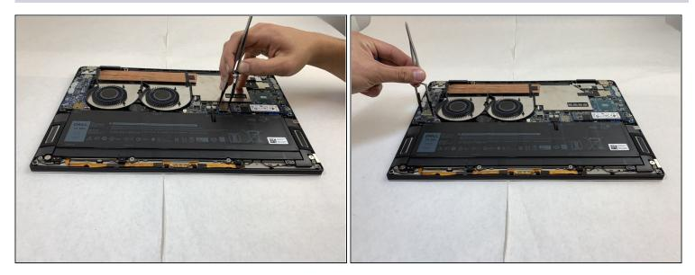
• Use the nylon <u>tweezers</u> to remove the interconnect pins from each of the circuit boards.
