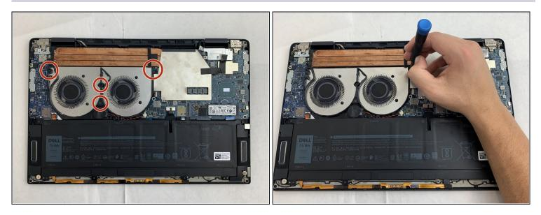
• Use the Phillips 0 Screwdriver to carefully extract each of the four 3.2 mm screws.
