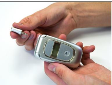
Rotate the antenna counter-clockwise until the antenna is completely removed.
