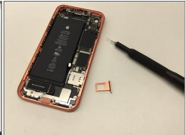
Use a SIM tool to remove the SIM tray.
