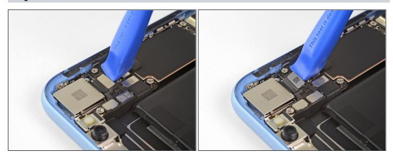
• Use an opening tool or fingernail to disconnect the camera cable connector by prying it straight up from its socket.
