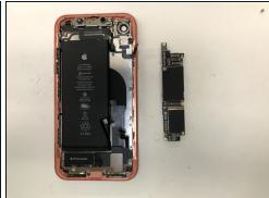
• Pull the logic board from the rear housing.
