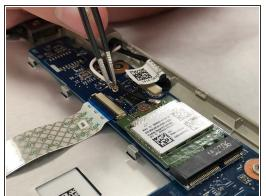
Remove the foam and unplug the black and white coaxial cables to the network card by pulling upward using the black tweezers.
