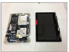
Open the laptop and remove the display assembly from the keyboard assembly.
