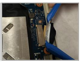
Unplug the power connector by pulling back the tape and sliding the connector away using the blue opening tool.
