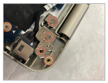
Using a Phillips #1 screwdriver, remove four 5.00 mm screws from both corner hinges of the display assembly.
