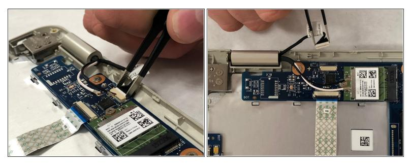
Remove the black webcam connector by pulling backwards with the tweezers.
