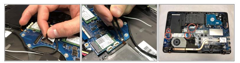
• Lift the connecting ports up prior to removing the connectors.
