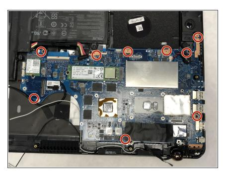
• Remove nine, 3.2 mm screws to fully release motherboard.
