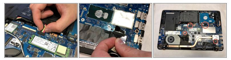
• Disconnect the four marked cables connectors at the sockets.
