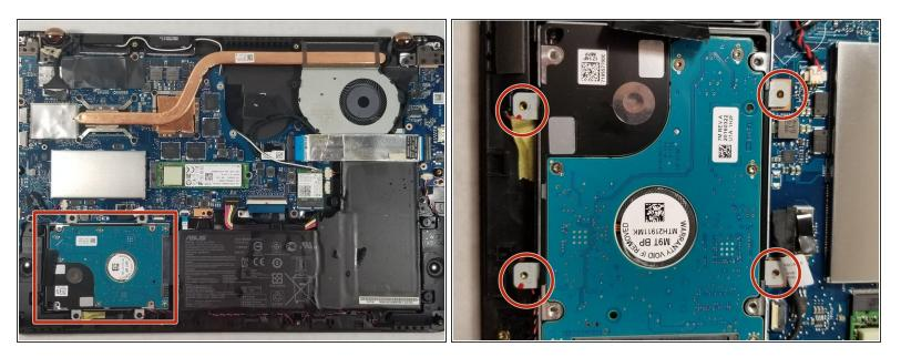
Remove four screws with the Phillips #00 screwdriver.
