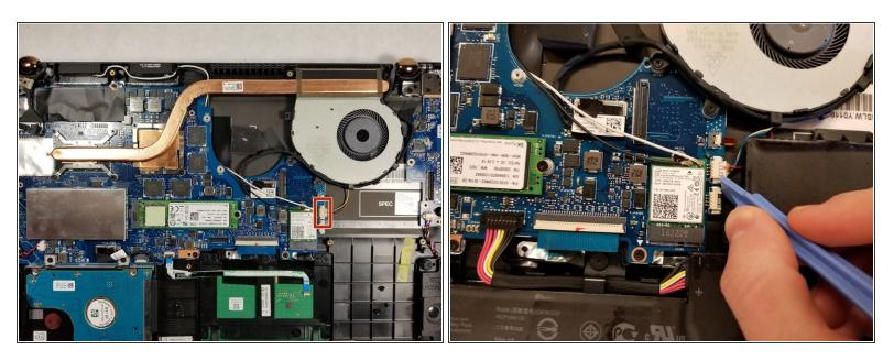
• Using the iFixit opening tool, gently pry the CPU fan connector out of the socket.
