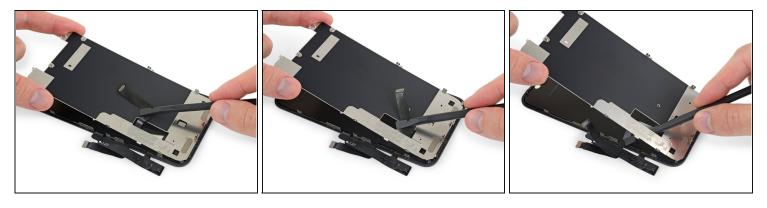
• Raise the top edge of the LCD shield a bit higher, and feed the rest of the display cable through the cutout in the shield.
