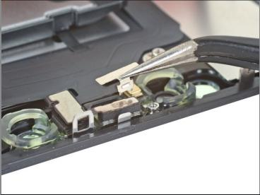
• Use <u>tweezers</u> to slide the small bracket straight up and off of the ambient light sensor.
