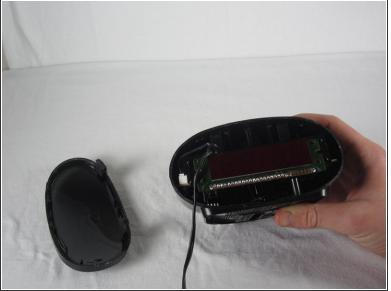
Using a moderate amount of force, position the screwdriver in the crack between the front screen and the main body of the clock (as shown) and push the screen away from the main body of the clock. To reassemble your device, follow these instructions in reverse order.
