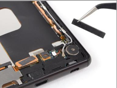
Use a pair of tweezers to peel off and remove the foam pad on top of the daughterboard.
