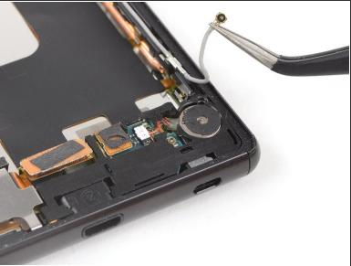
• Use a pair of tweezers to pry up and disconnect the antenna cable.
