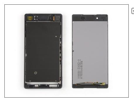
Remove any remaining adhesive from the midframe, and clean the glued areas with isopropyl alcohol and a lint-free cloth before installing a new screen.
