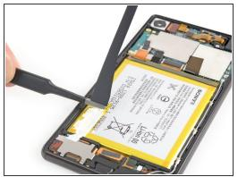
Use a pair of tweezers to carefully peel the adhesive strip off the mother board and the battery and remove it.
