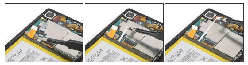
Repeat the previous process with the adhesive tab next to the battery flex cable.
