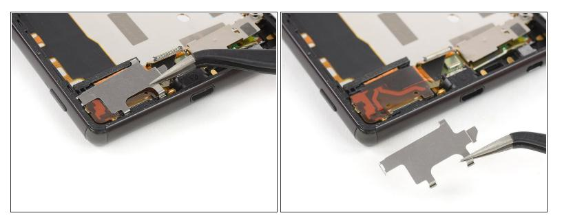
Unhook and remove the metal shield above the loudspeaker cover located at the bottom left.
