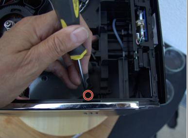
• The left side is still attached via two Torx T10 screws at the top. Remove them.
