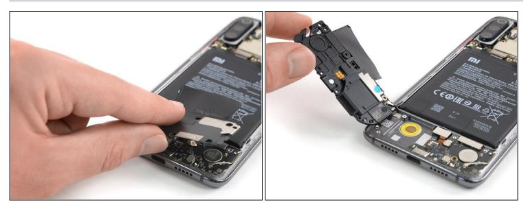
$\triangle$  There is still an antenna cable connected to the back of the unit.
