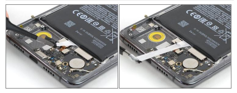
• Use a pair of tweezers to pull out the right adhesive tab from underneath the battery.
