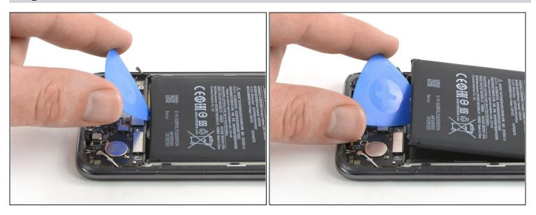
• Use an opening pick to pry the battery out of its recess until you can get a good grip.
