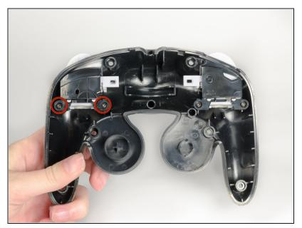
• Remove the two 8.9mm Phillips Head #0 screws.
