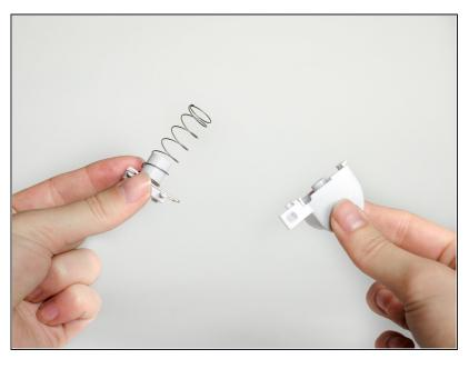
• Pull the metal clip from the trigger.
