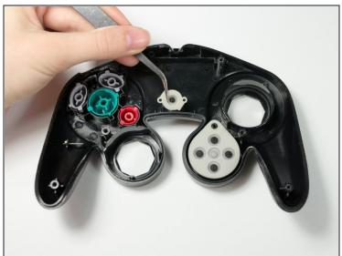
• Remove the rubber backing that covers the buttons.
