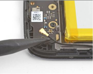
Use the point of a spudger to pry up and disconnect the antenna cable from its daughterboard socket.
