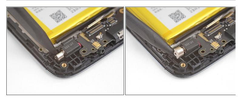
• Insert the point of a spudger underneath the vibration motor and pry upwards to loosen it.
