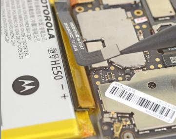
Use the point of a spudger to pry up and disconnect the battery connector from its motherboard socket.
