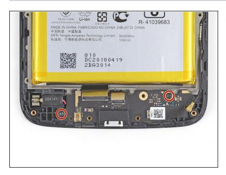
Remove the two 3.2 mm long T3 screws securing the daughterboard.
