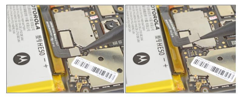
• Use the point of a spudger to pry up and disconnect the battery connector from its motherboard socket.
