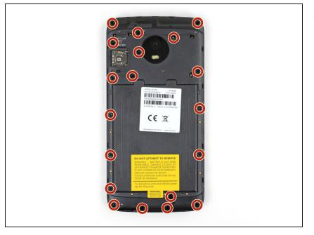
Remove the nineteen 3.2 mm long T3 screws securing the plastic midframe.
