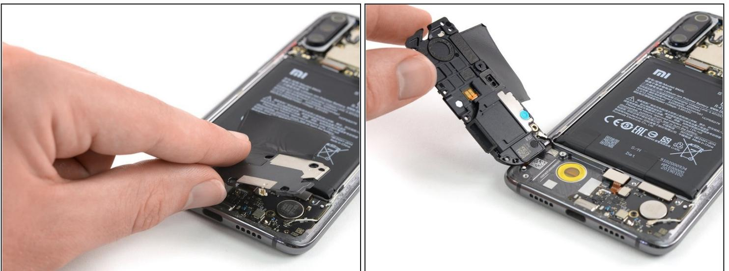
**⚠ There is still an antenna cable connected to the back of the unit.**
