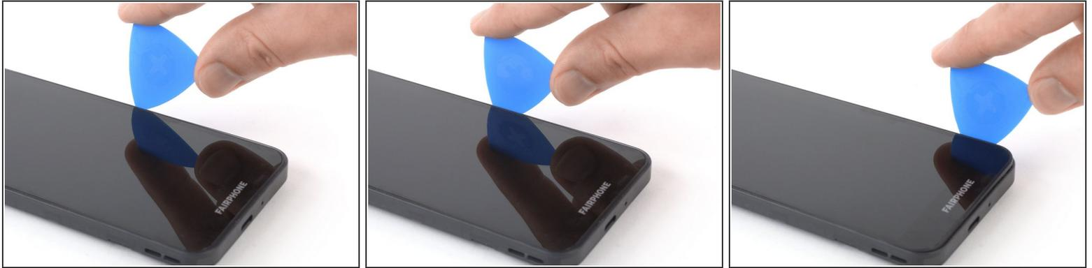
**⚠** Make sure to insert the opening pick between the midframe and the display module and not into the small gap next to the screen. Otherwise you're going to pry up the screen instead of the whole display module.
