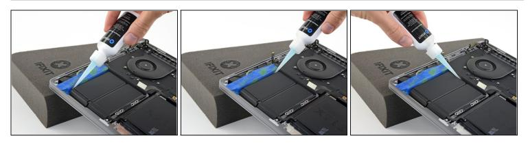
• Apply a few drops of adhesive remover under the far left battery cell, and wait about two minutes for it to penetrate.
