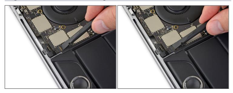
• Flip open the locking flap for the left main speaker ZIF connector by prying it straight up from the logic board.
