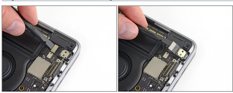
Use a spudger to disconnect the Touch Bar digitizer by prying its connector straight up from the logic board.
