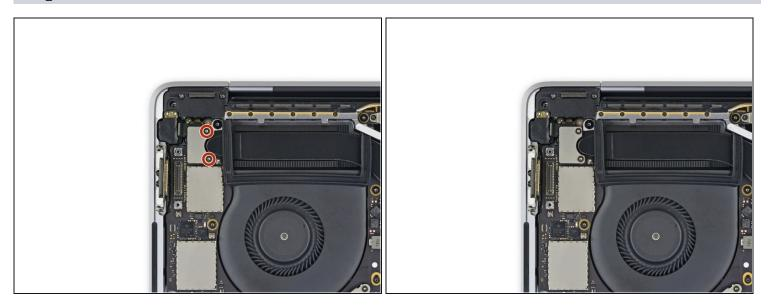
• Use a T3 Torx driver to remove the two 1.9 mm screws from the cover bracket securing the Touch ID and 3.5 mm audio jack connectors.
