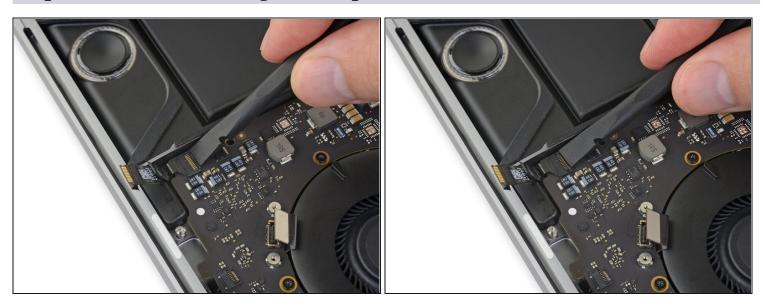
• Flip open the locking flap for the right-side main speaker ZIF connector by prying it straight up from the logic board.
