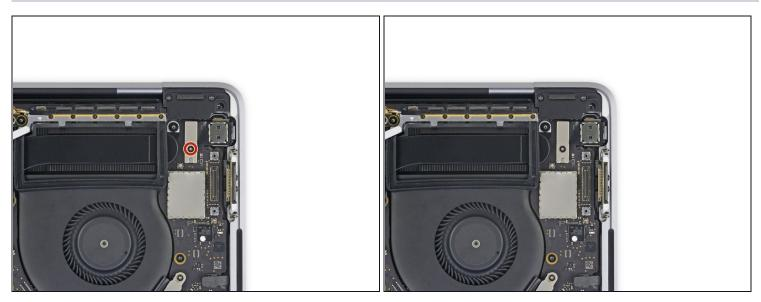
Use a T3 Torx driver to remove the 1.9 mm screw from the Touch Bar digitizer connector bracket.
