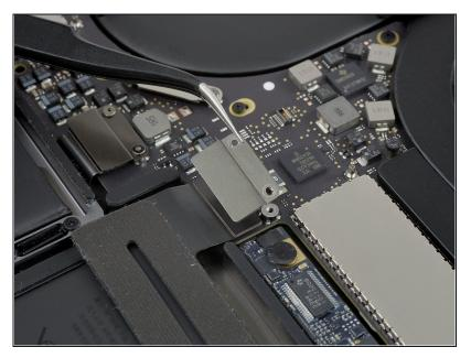
Remove the trackpad cable connector bracket with a pair of tweezers.
