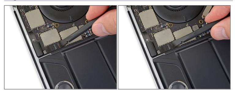
• Flip open the locking flap for the left-side tweeter ZIF connector by prying it straight up from the logic board.
