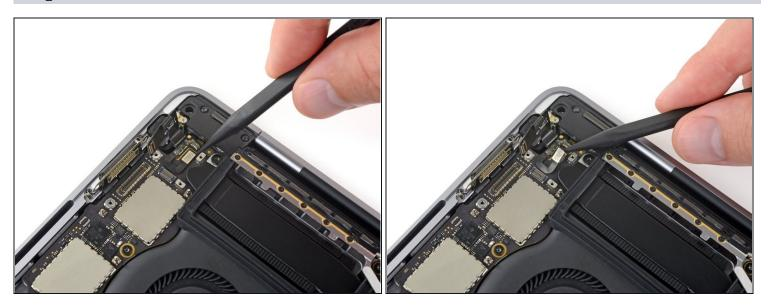
• Disconnect the Touch ID and power button flex cable by prying it straight up from the logic board.
