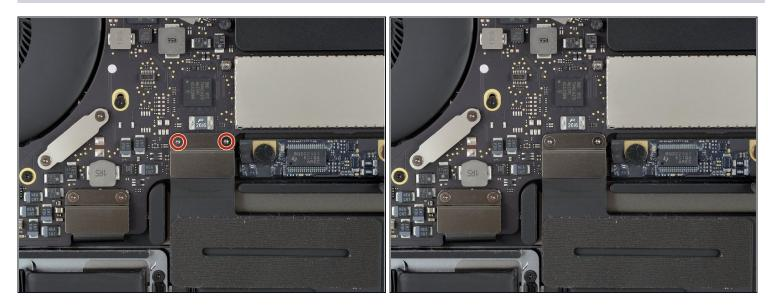
• Use a T3 Torx driver to remove the two 1.8 mm screws securing the trackpad cable connector bracket.
