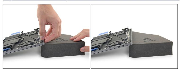
• Next, raise the back edge of your MacBook Pro to direct the flow of adhesive remover away from the keyboard/logic board area.
