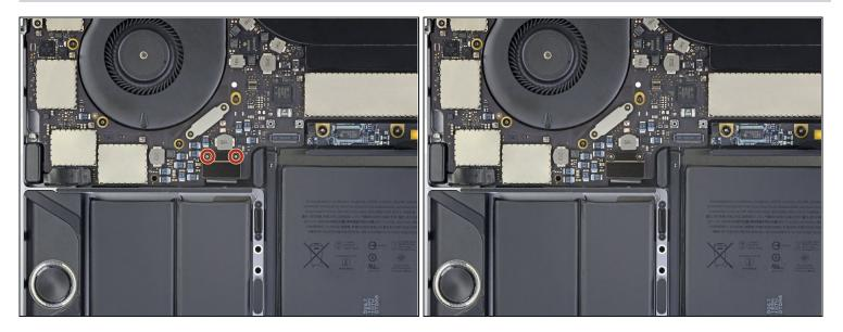
• Use a T3 Torx driver to remove the two 1.9 mm screws from the keyboard connector bracket.
