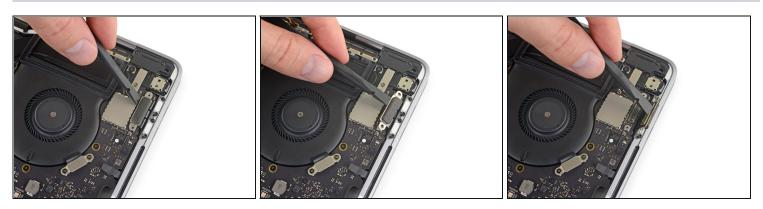
• Repeat for the right-side Thunderbolt port connector, prying it up from the inside edge and pushing it carefully aside.
