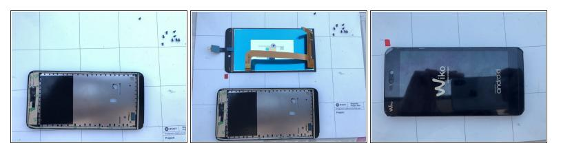
Apply the double sided tape on the edges of the frame so the enclosure is ready for a new display.
