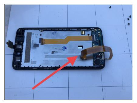
Remove the flat cable interconnecting the display and the motherboard. It's glued on the back of the frame.
