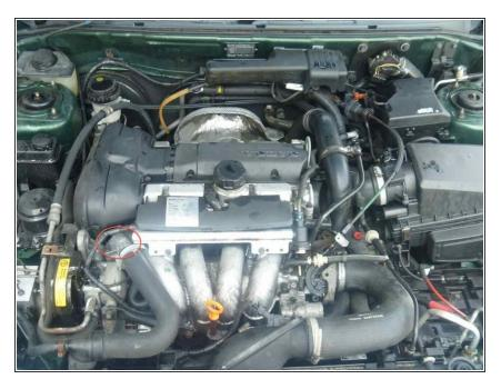
Locate the two bolts that secure the inlet to the engine block and remove them. Use a 12 mm socket and ratchet. Pull the water inlet off the engine block. Due to age, the inlet may stick to the block. Place pressure on the side of the inlet to break the seal, if needed.
