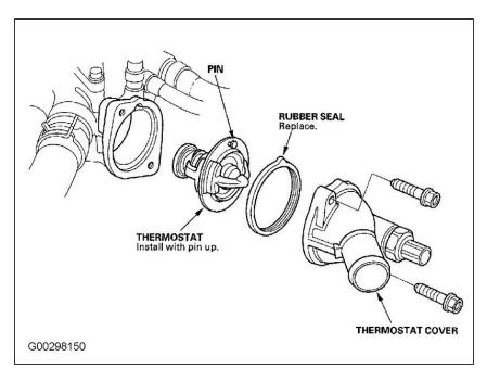
Pull the old thermostat out of the engine and place the new one into the engine. One end of the thermostat has a large spring. The spring sits inside of the engine.
