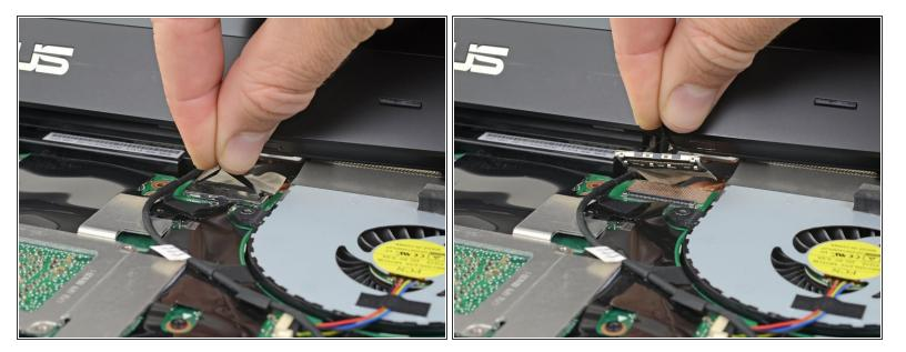
Grab the black tape attached to the display cable and pull straight up to disconnect the display cable.
