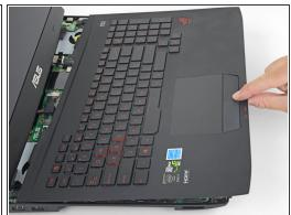
When all the clips securing the upper case assembly have been released, lift the assembly slightly and slide it down, away from the display, about an inch.
