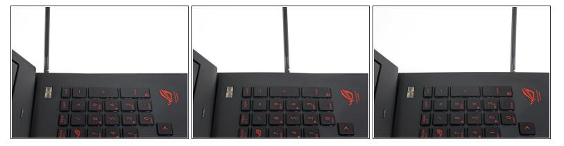
Slide the spudger along each edge of the upper case assembly, prying and releasing clips as you go.
