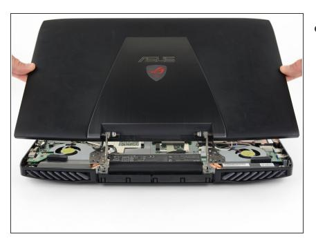
Lift the monitor straight up and remove it.
