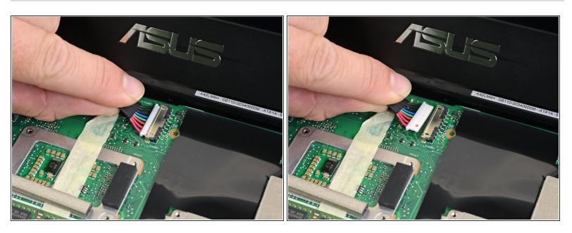
Pull the battery cable away from the connector in the same direction as the individual wires are running to disconnect the battery.
