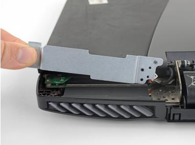
Lift up and remove the two metal display brackets.
