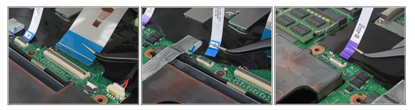
Repeat the previous step for the keyboard, trackpad buttons, and trackpad cables held in place by ZIF connectors.
