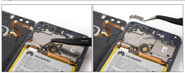
• Use a pair of <u>tweezers</u> to remove the metal bracket that sits on top of the fingerprint and display flex connectors.
