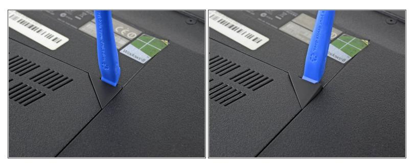
Use an opening tool to pry up the small rubber cover on the upper right corner of the RAM access door.
