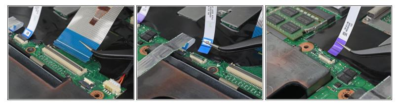
Repeat the previous step for the keyboard, trackpad buttons, and trackpad cables held in place by ZIF connectors.
