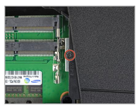
Remove the 5.2 mm Phillips #00 screw securing the optical drive.
