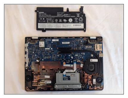
• Lift the battery out of the upper case.
