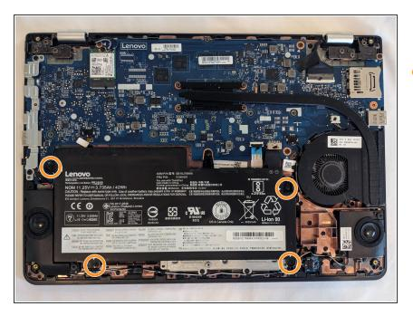
Remove the four screws securing the battery to the upper case.
