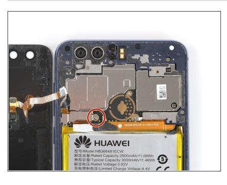
Remove the Phillips #00 screw (2.8 mm length) that secures the metal bracket on top of the fingerprint flex connector.
