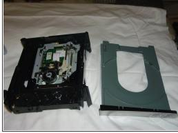
Clean the runners where the tray slides with rubbing alcohol as well. If it is really filthy like this one, you may want to remove the tray for a more thorough cleaning. Release the tab shown and pull the tray out and to the side.
