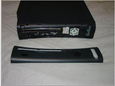
• The next step is to remove the face plate. Pull out on the right side of it (by the USB cover). There are clips that hold it in place, you just need to pop it loose.
