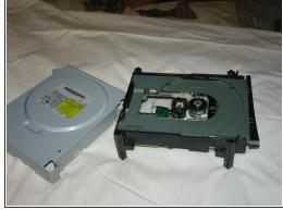
Remove the screws and cut or peel the security sticker on the side of the DVD drive (also voids the warranty). Lift off the bottom and top metal case.
