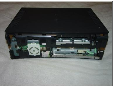
To open the front you will need to cut or peel back the Microsoft sticker. THIS WILL VOID ANY WARRANTY ON THE XBOX. Turn xbox upside down, release the four clips shown, and lift the front of the bottom cover.
