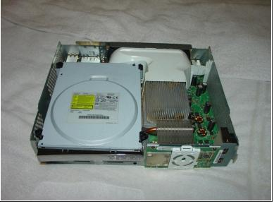
There are six #10 Torx screws that hold the upper case on. Remove these, turn the xbox over, and lift the top cover off.
