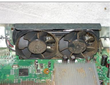
Now is a good time to blow the dirt out. The fan shroud has a clip in the center, you can release that with the finger of the xbox tool and lift it straight up. The fans have two clips, one above each fan, lift up on the metal lip to release them. Don't forget to unplug the electrical connector also. Clean it out and re-assemble these parts.
