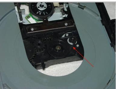
To open your tray, look under the front of it. There is a small wheel that you can use the finger of the xbox tool to rotate by pulling from right to left. (In other words, rotate clockwise as seen from above.) This will lower the laser assembly and allow you to slide the tray. Clean the rubber belt with rubbing alcohol, or replace if necessary.
