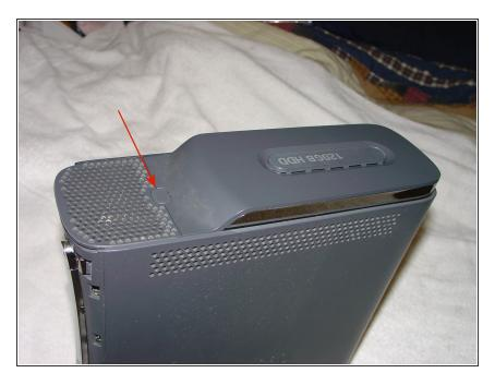
The first step is to remove the hard drive if one is installed. Push the button at the front of the hard drive and lift the hard drive up to remove it.
