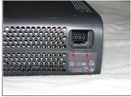
• Use the xbox tool to release the five points under the serial number label and start to lift the cover from that side. There is a clip in the middle you also may need to release. Then use the xbox tool to release the last two points at the power connection. Lift the bottom cover off the xbox.
