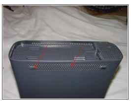
• The other vent has two holes towards the front of the xbox. Slide the finger of the xbox tool or the pointed end of the spudger into these holes to release the front two clips. There are two additional clips that are release from the sides, lift from the front as you release those clips. The back clip on the bottom is under the rubber "foot".
