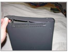
Next we will remove the bottom vent cover. There are three tabs on each side, use the finger of the xbox tool or the pointed end of a spudger to release them one at a time, and pull up from the front as shown in the third pic.
