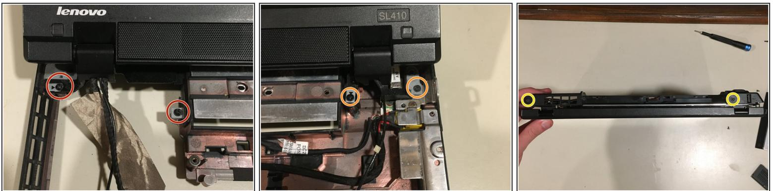
**⚠** During this step, be careful that the display does not fall backwards, which could potentially cause damage.
