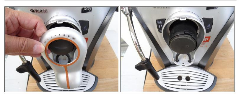
Remove the cover from the coffee spout. Lift them from bottom to top, using only plastic tools to pry.
