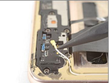
• Use the point of a spudger to pry up and disconnect the white antenna cable from the bottom of the phone.
