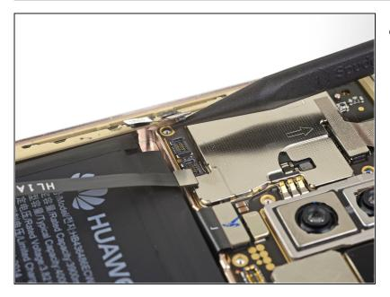
Use the point of a spudger to pry up and disconnect the button connector from its motherboard socket.
